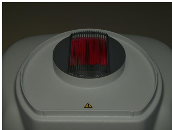
Figure 41: 0.25ml IMV straws positioned on H01 head
